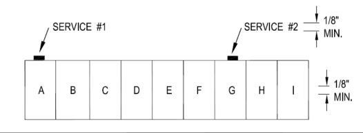
The plaque or directory shall be manufactured in metal or plastic, suitable for the environment, with engraved or machine-printed lettering or electro-photo-plating in a contrasting color. The plaque shall include a properly oriented footprint of the entire building, properly oriented, with the area served by each service clearly delineated. The plaques shall be located at the service disconnect and securely fastened by permanent means acceptable to the AHJ.
